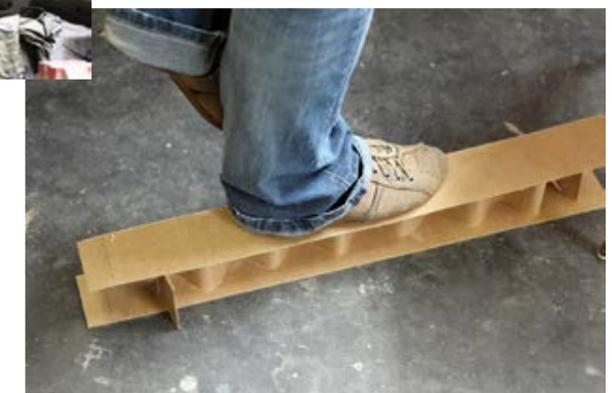
Kraftplex is made of pure wood fibers but is still stiff, flexible, and formable like metal sheeting - this versatile material is also called "Wooden Sheeting". Processing and experiments: Moisturizing, heating, cutting, wire pressing, glueing, deep drawing, bending, tearing, turning, painting, waxing, oiling, pressing, laser cutting, covering, perforating ...
