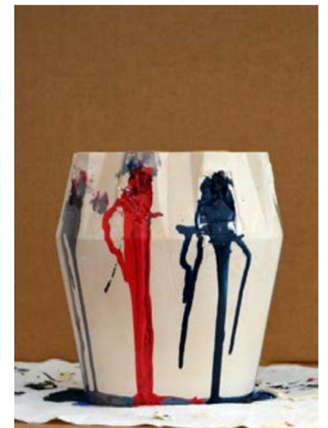
Acrylic One: is a two-component material consisting of a mineral powder and a water based acrylic resin. These bond and result in a very strong material. It can be molded, laminated or sprayed. The result is non-toxic, fire resistant, and can be painted or further processed (drilling, milling, polishing, etc.).
